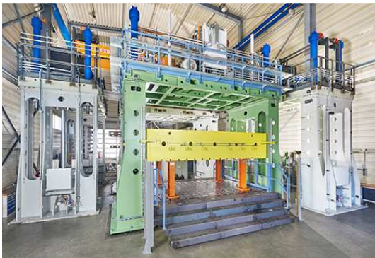
Image 2: The lifting frame does not need an extensive press pit and can be flexibly disassembled and set up again elsewhere. (Copyright: Bosch Rexroth AG)
